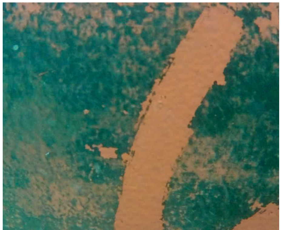
Demonstration of low adhesion of fouling on durable hard coating
