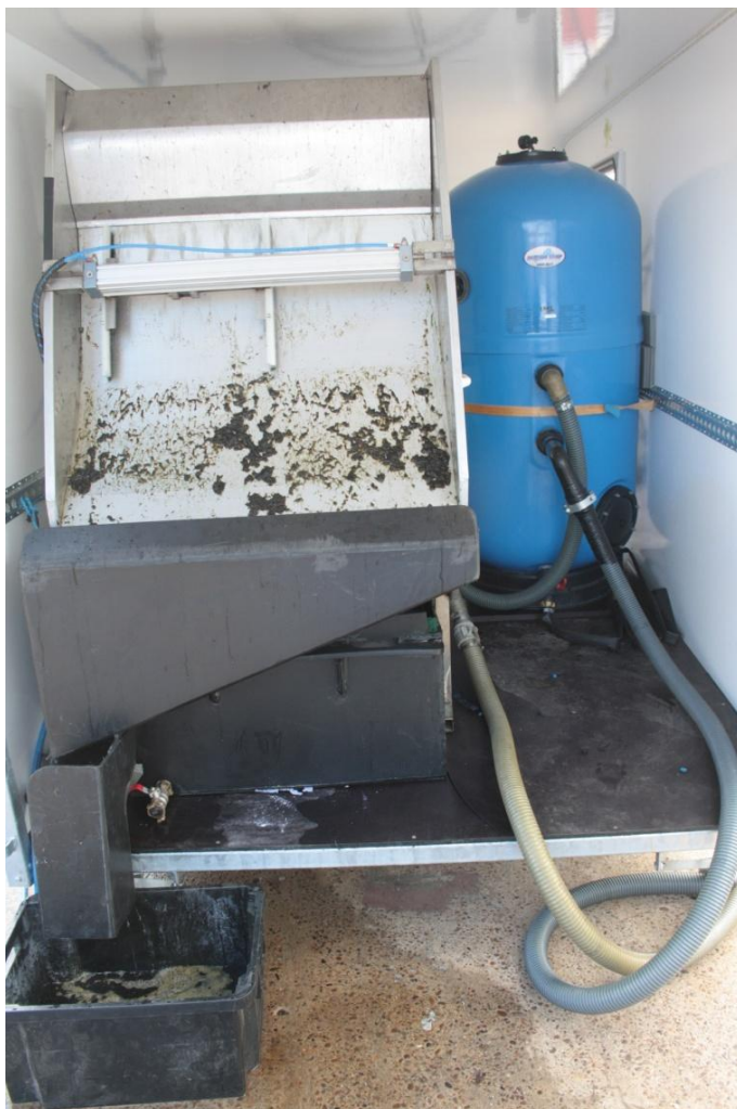
Fig. 33: Water treatment unit with thief filter (100 µm pore size) above a fleece filter (100 µm pore size) with grey tube releasing the treated water back into the harbour basin.
