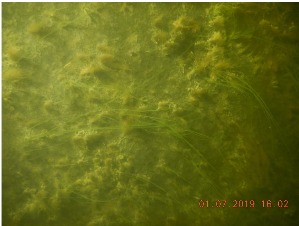
Fig. 6: Fouling community composed of biofilm and filamentous green algae, aft, „Polarstern“ at July 1, 2019 before the underwater cleaning by DG Diving
