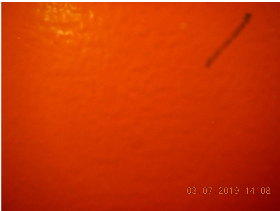
Fig. 20: Cleanable hard coating of Jotun, ,Wega', July 2019 with heavy macrofouling mainly composed of filamentous algae and barnacles, after cleaning, DG Diving
