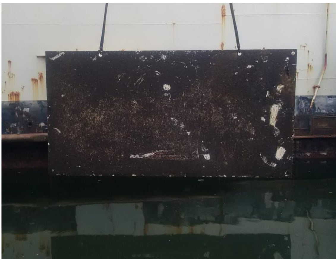
Fig. 45: Steel panel after 7 months of static exposure, before cleaning
