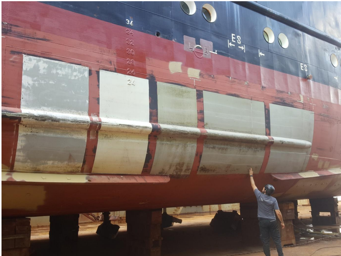
Fig. 32: Test patches of foul release coatings, ,Wega', July 2019, after hp-washing in dry dock
