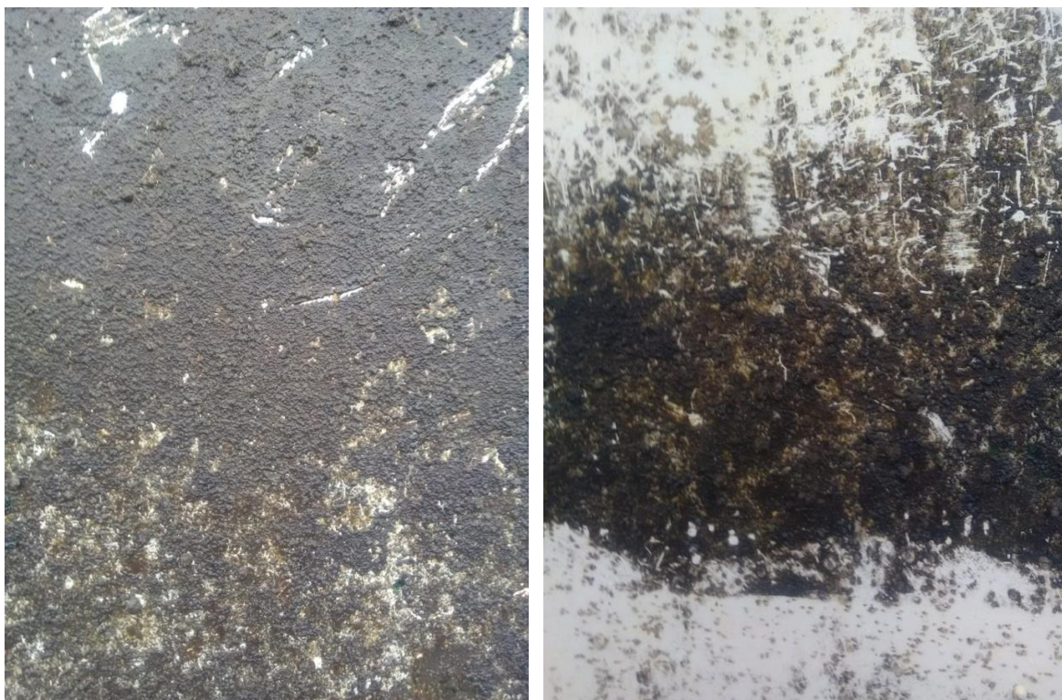
Fig. 44: Fouling on steel panel after 7 months of static exposure Bredo-Dockyards, Bremerhaven
