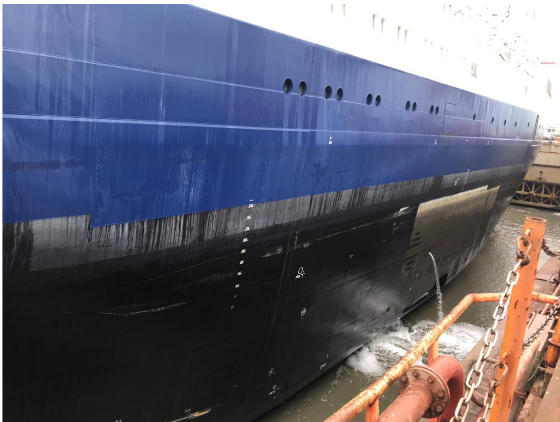
Fig. 11: RV 'Polarstern' after underwater cleaning in the dry dock (Lloyd Dockyards, Bremerhaven), July 2019
