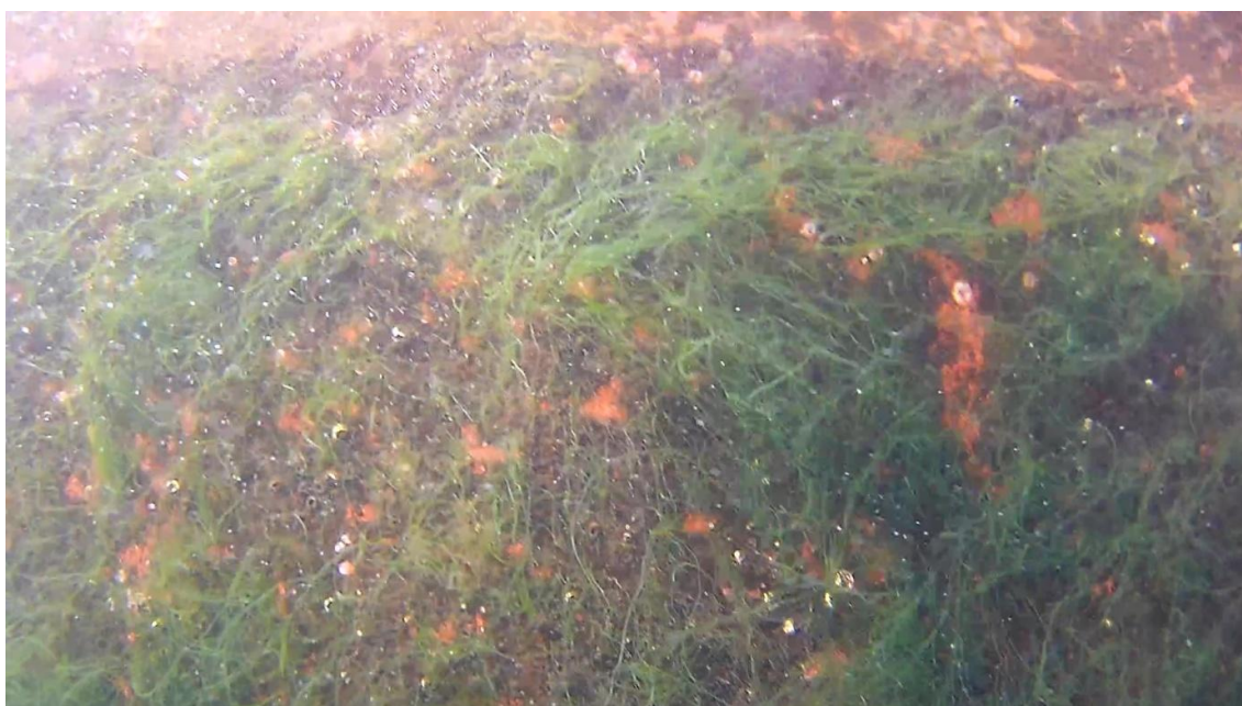
Fig. 16: Cleanable hard coating of Jotun, 'Wega', April 2019 with heavy macrofouling mainly composed of filamentous algae and barnacles, before cleaning, Wega diving crew
