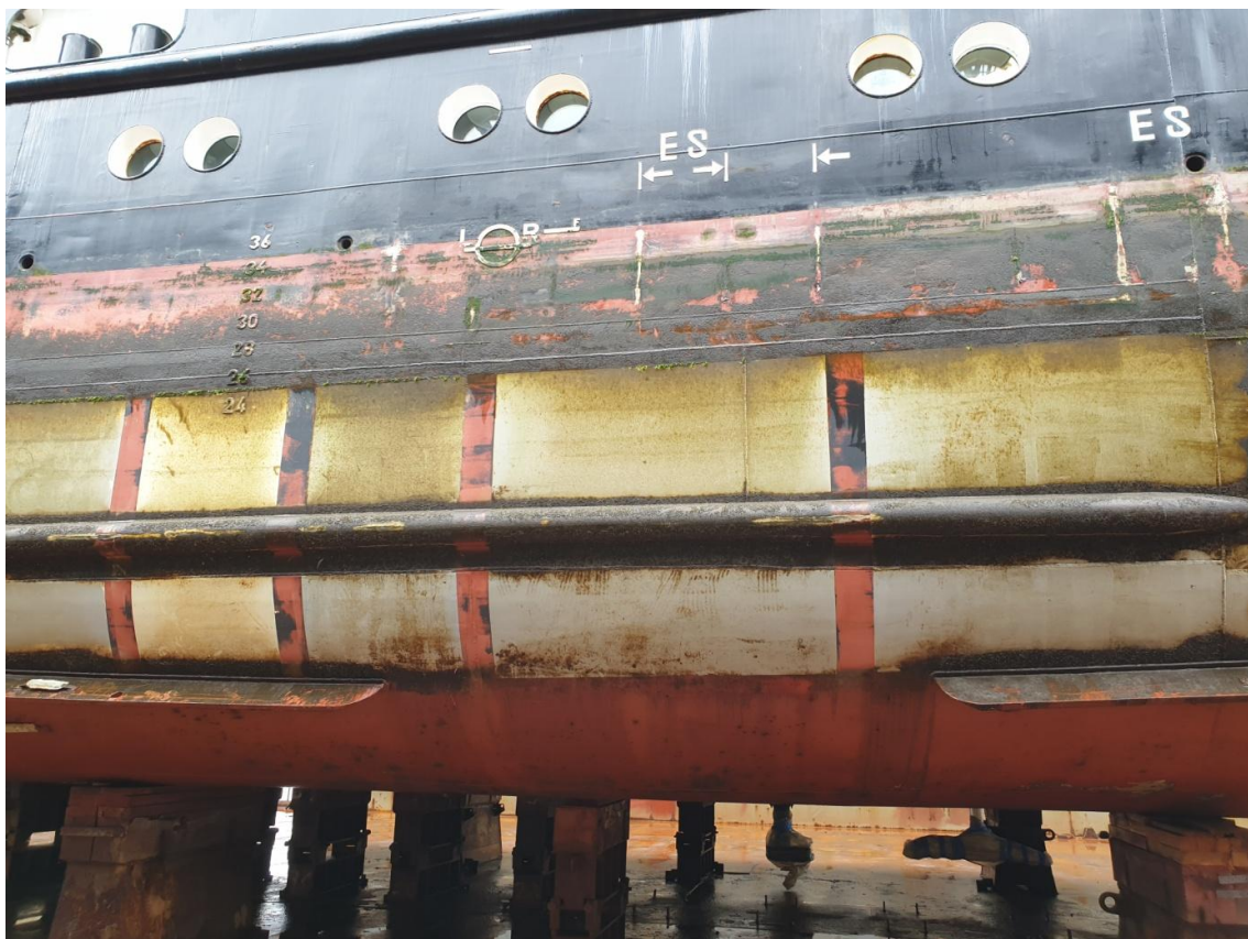
Fig. 31: Test patches of foul release coatings, ,Wega', July 2019, after underwater cleaning
