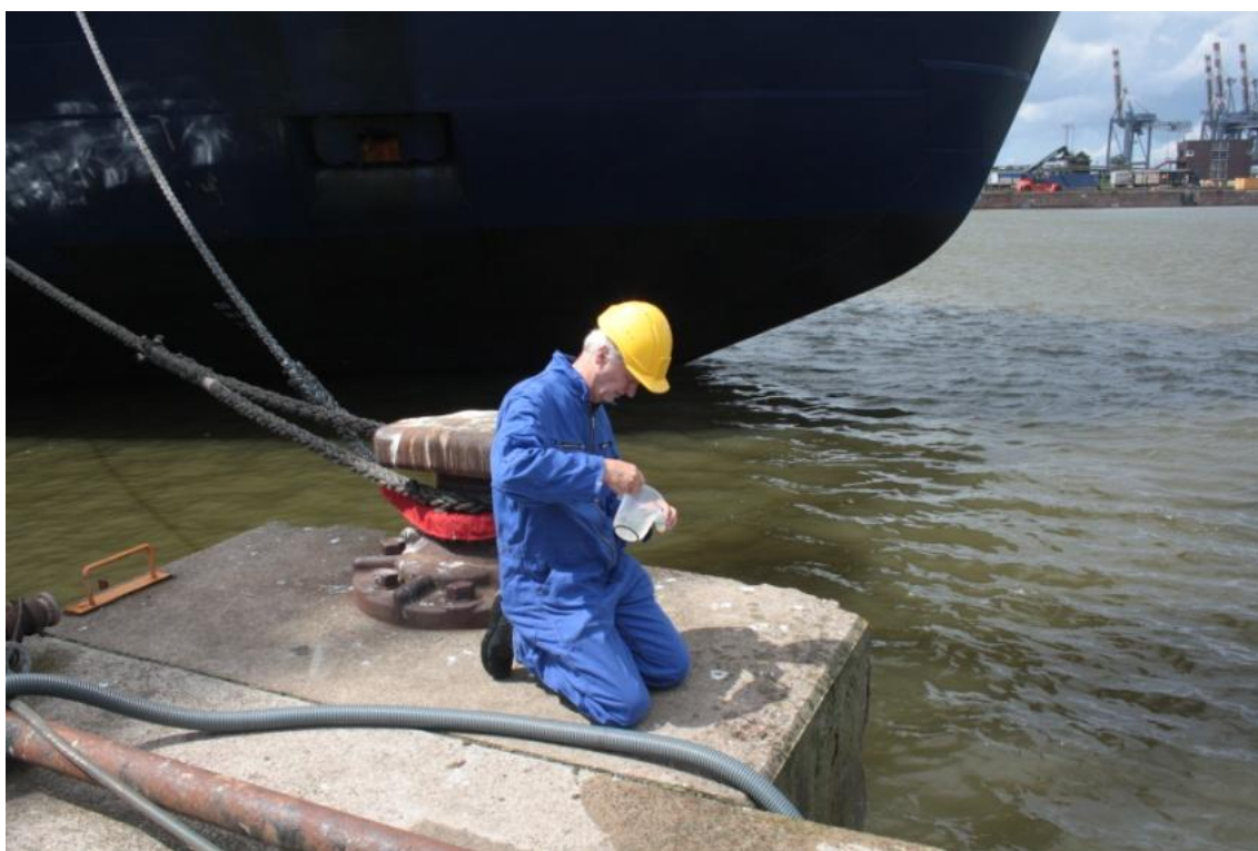
Fig. 34: Water sampling at the effluent tube of the water treatment unit
