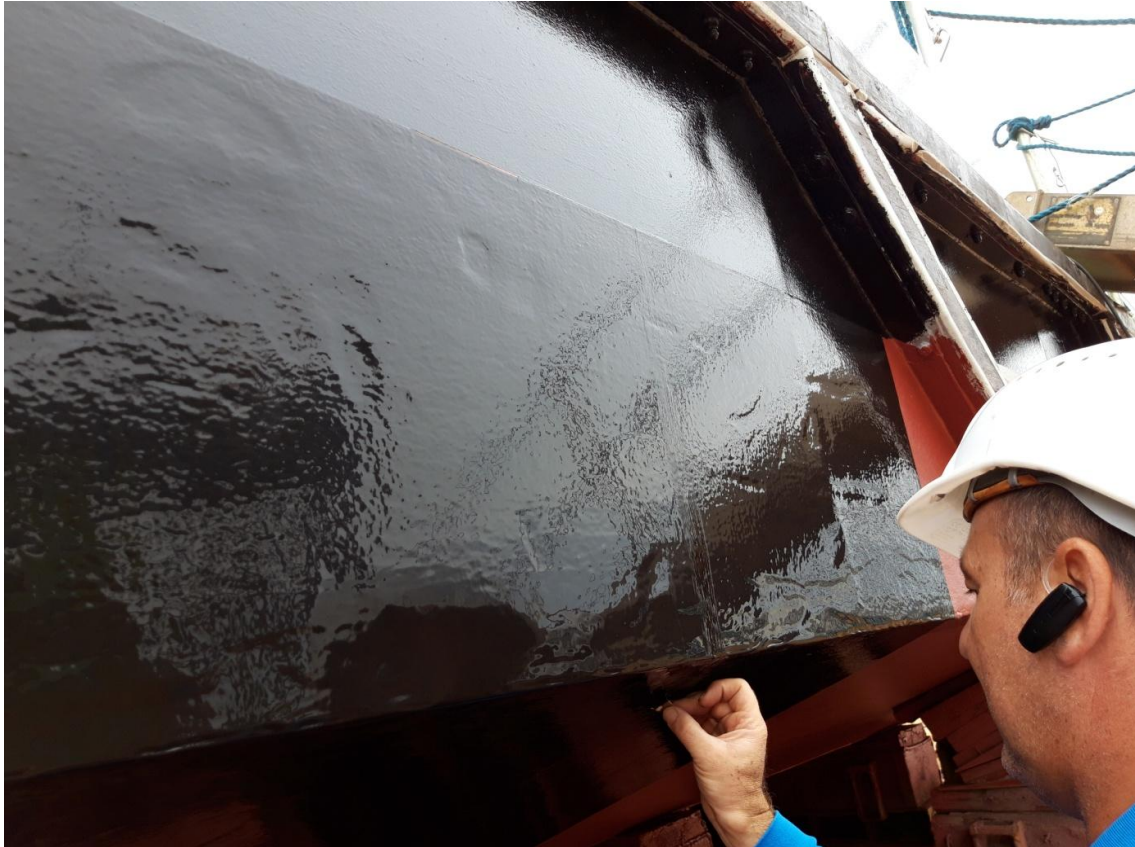
Fig. 40: Foul release adhesive film ,Dolphin S', mis ships ,MÖWE' during application August 2019
