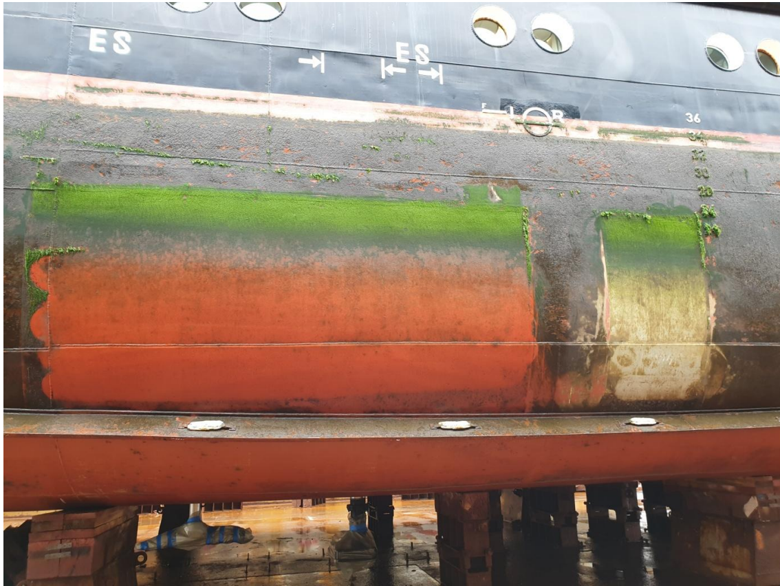
Fig. 21: Cleanable hard coatings, portside ‚Wega‘, test patches left Jotun, right Momentive/Wohlert, July 2019
