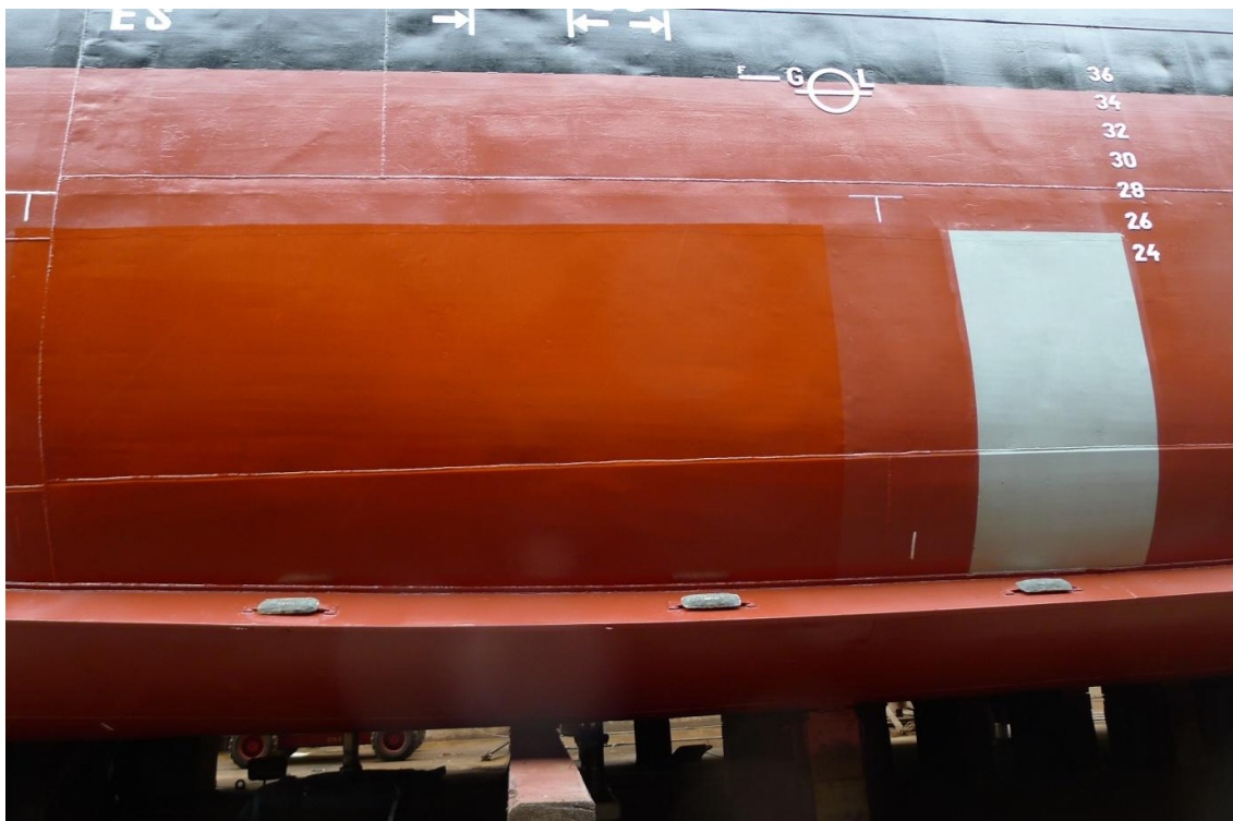
Fig. 15: Cleanable hard coatings, portside 'WEGA', after application, November 2015
