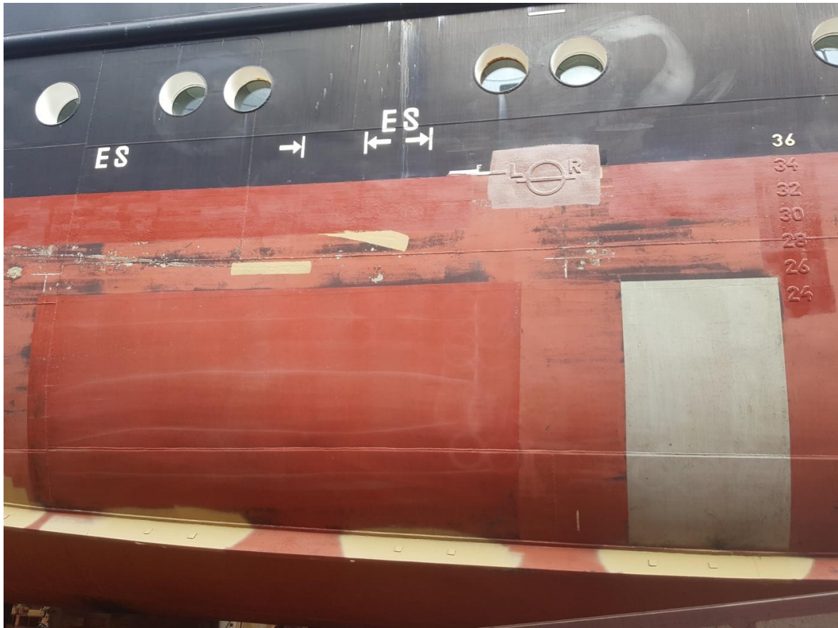
Fig. 27: Cleanable hard coatings, portside, 'Wega', after hp washing in the dry dock, July 2019, left Jotun, right Momenitive/Wohlert
