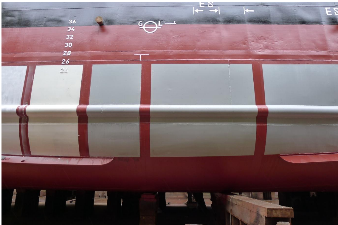
Fig. 28: Foul release coatings on starboard after application November 2015, 'Wega'
